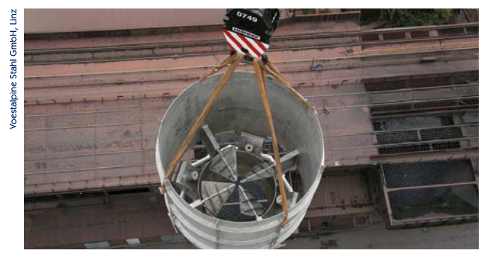
Flare stack burner with twist counter and pilot burners
