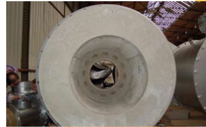
Air baffle of a sinter burner
