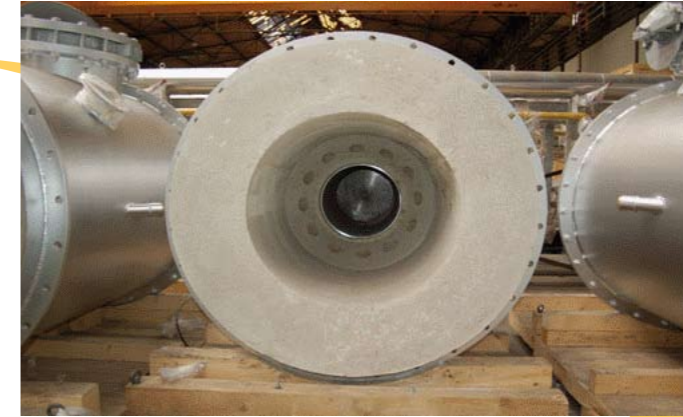
Burner for coke oven gas 8 MW
